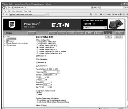
Quick Setup (Power Xpert Meter 4000/6000/8000)
